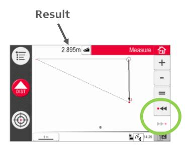
Measured points are connected with a line. Use scroll keys or tip on the sketch to select one. You find more results like angles, tilt, height difference etc. behind this key:
