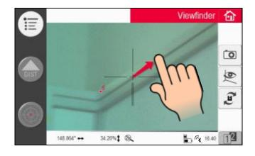
Glide to any direction. The laser follows until you release the screen.
