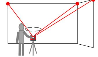
Turn the laser spot to the positions you want to measure and press DIST.
