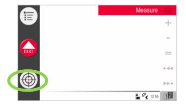
Press the "Viewfinder" key. Camera and laser switch on.
